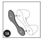
Be sure to keep rubber gasket in place when installing the DUO. see image 1A.
