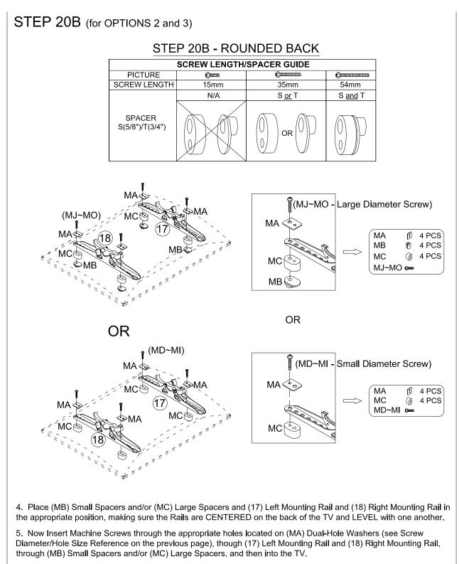
\*NOTE: the position of the Mounting Brackets and Hardware will be determined by the type of TV that you have. These diagrams are not designed to show the exact positioning, they are only to be used as a guide.
