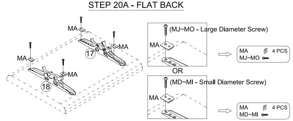
3. Now Insert Machine Screws through the appropriate holes located on (MA) Dual-Hole Washers (see Screw Diameter/Hole Size Reference above), next though (17) Left Mounting Rail and (18) Right Mounting Rail, and then into the TV.
