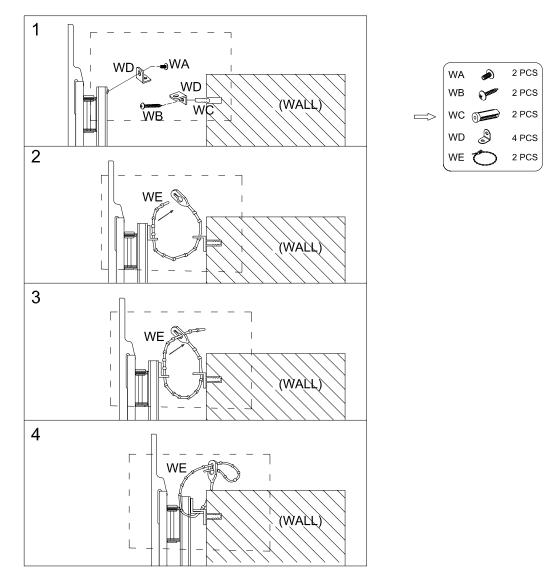
1. Attach (WD) Mounting Tabs to the BACK of the Product with (WA) 4.5 x 10 x 8mm Machine Screws, making sure the Tabs extend DOWNWARD as shown.
