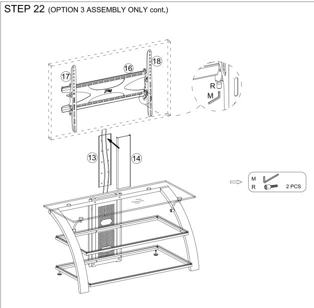
1. Carefully set (17) Left Mounting Rail and (18) Right Mounting Rail onto (16) Upper Mounting Panel, making sure that the rail hooks over the TOP edge of the Mounting Panel. Tighten (R) Adjustable Screw on (17) Left Mounting Rail and (18) Right Mounting Rail using (M) Long Allen Wrench as shown.
