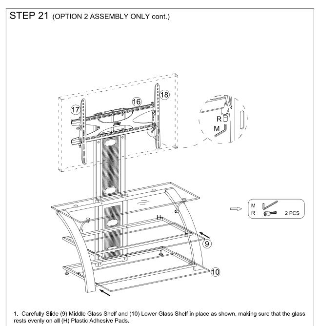
2. Carefully set (17) Left Mounting Rail and (18) Right Mounting Rail onto (16) Upper Mounting Panel, making sure that the rail hooks over the TOP edge of the Mounting Panel. Tighten (R) Adjustable Screw on (17) Left Mounting Rail and (18) Right Mounting Rail using (M) Long Allen Wrench as shown.
